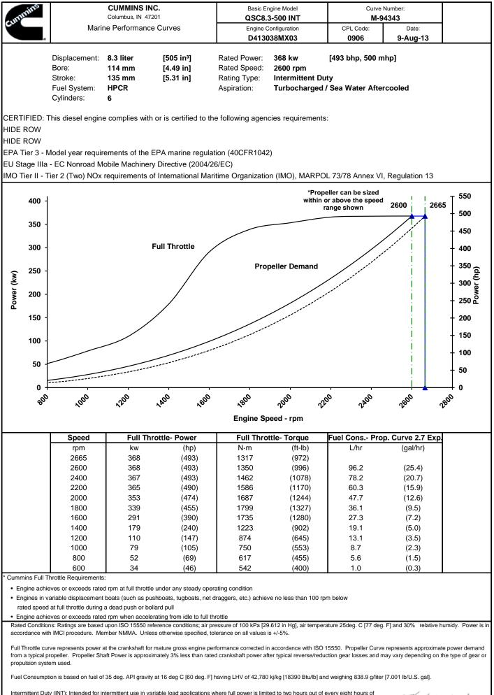
Intermittent Duty (INT): Intended for intermittent use in variable load applications where full power is limited to two hours out of every eight hours operation. Also, reduced power operations must be at or below 200 rpm of the maximum rated rpm. This rating is an ISO 15550 fuel stop power rating and is for applications that operate less than 1,500 hours per year.
