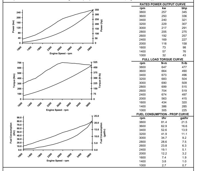
Rated Conditions: Ratings are based upon ISO 8665 and SAE J1228 reference conditions; air pressure of 100 kPa [29.612 in Hg], air temperature 25deg. C [77 deg. F] and 30% relative humidy. Power is in accordance with IMCI procedure. Member NMMA.
