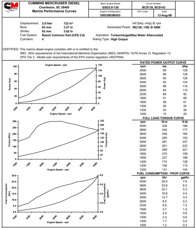
Rated Conditions: Ratings are based upon ISO 8665 and SAE J1228 reference conditions; air pressure of 100 kPa [29.612 in Hg], air temperature 25deg. C [77 deg. F] and 30% relative humidy. Power is in accordance with IMCI procedure. Member NMMA.
